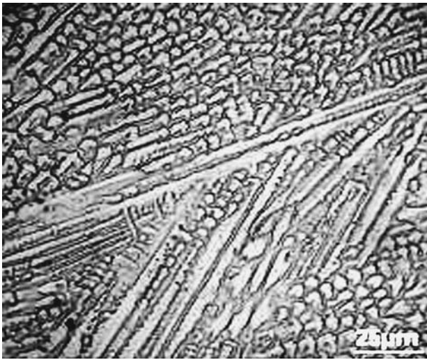
Fig. 8 Micrograph of weld zone adjacent to fusion boundary showing cellular-dendritic morphology of grains
